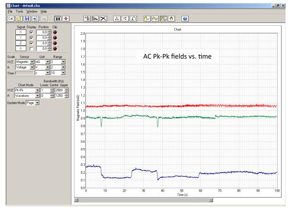
When charting the magnetic field waveform, the program is able to extend the low frequency limit of the AC magnetic field sensor by post-processing its output with a digital filter that boosts the low frequencies. The 1/f noise of the sensor is also boosted by the same amount and this sets a limit to the usefulness of this feature. With the low frequency set to 0.1Hz the 1/f noise is about 0.2mG Pk-Pk which is small enough to distinguish typical tram fields from the noise.
