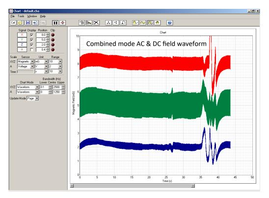
The waveform chart below has the bandwidth set to 0.1 Hz - 1.0 Hz to show only the slowly changing field from trams. If true DC field measurement is required the optional MEDA  $\mu$ MAG-01N magnetometer should be used.
