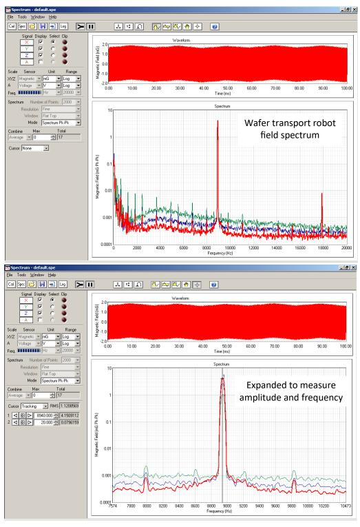
Tracking cursors are provided to measure features of the spectrum as well as define bands for RMS measurement. Harmonic cursors can be used to recognise harmonics in the spectrum and enable more accurate measurement of the fundamental frequency. Successive spectra can be combined over a period of time, as an average to reduce noise, or to find the worst case peak values. Spectra can be data-logged to a file at a maximum rate of once every minute to trace sources that vary.
