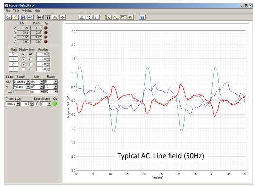
The oscilloscope has a bandwidth of 20kHz on its shorter time ranges. The A input is DC coupled. There are common controls for the time base and the magnetic field axis ranges. There are independent controls for the auxiliary channel range and the vertical position of each channel. The RMS and Pk-Pk values of the waveforms are measured and displayed numerically.
