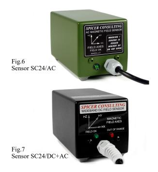
that surround its field sensing elements. They are used to offset the DC component of the ambient field including the earths field. At reset, the microcomputer in the sensor adjusts and remembers the currents in the coils to set the X, Y, Z sensor outputs to zero. The reset process takes 1 second. The sensor must be reset if it is moved.
