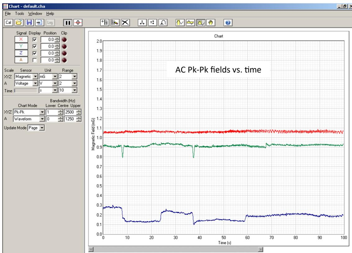
When charting the magnetic field waveform, the program is able to extend the low frequency limit of the AC magnetic field sensor by post-processing its output with a digital filter that boosts the low frequencies. The 1/f noise of the sensor is also boosted by the same amount and this sets a limit to the usefulness of this feature. With the low frequency set to 0.1Hz the 1/f noise is about 0.2mG Pk-Pk which is small enough to distinguish typical tram fields from the noise.
