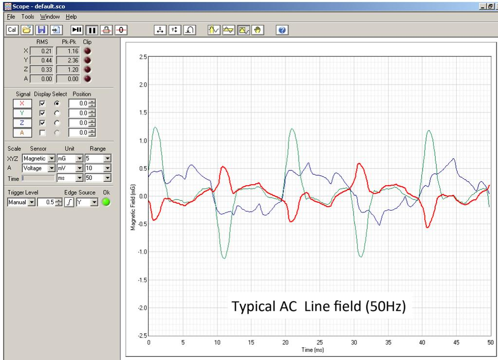
The oscilloscope has a bandwidth of 20kHz on its shorter time ranges. The A input is DC coupled. There are common controls for the time base and the magnetic field axis ranges. There are independent controls for the auxiliary channel range and the vertical position of each channel. The RMS and Pk-Pk values of the waveforms are measured and displayed numerically.
