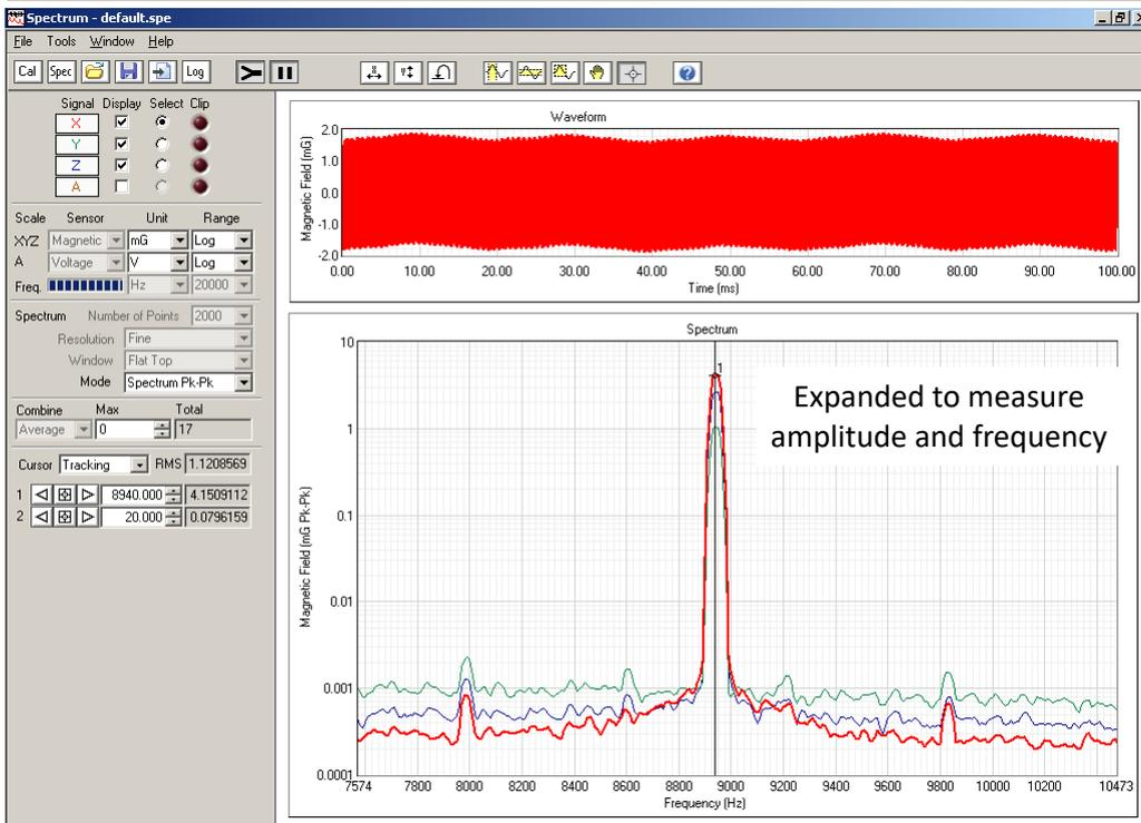
Tracking cursors are provided to measure features of the spectrum as well as define bands for RMS measurement. Harmonic cursors can be used to recognise harmonics in the spectrum and enable more accurate measurement of the fundamental frequency. Successive spectra can be combined over a period of time, as an average to reduce noise, or to find the worst case peak values. Spectra can be data-logged to a file at a maximum rate of once every minute to trace sources that vary.
