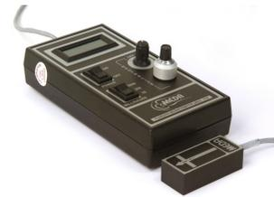
MEDA μMAG-01N magnetometer
