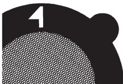
**600 Mesh Fine Bar: Pitch 42 $\mu$ m; Hole Width 37 $\mu$ m; Bar Width 5 $\mu$ m; Transmission 78%**
