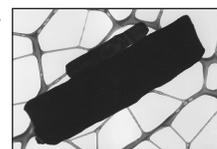
Molybdenum Trioxide Crystal on a Lacey Support Film, example of application
