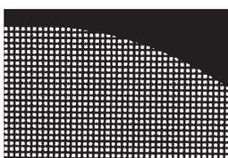
**1500 Mesh Fine Bar: Pitch 16.5 $\mu$ m; Hole Width 11.5 $\mu$ m; Bar Width 5 $\mu$ m; Transmission 49%**
