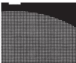
**2000 Mesh Fine Bar: Pitch 12.5 $\mu$ m; Hole Width 7.5 $\mu$ m; Bar Width 5 $\mu$ m; Transmission 36%**
